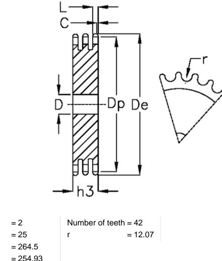
C = 2 D = 25 De = 264.5 Dp = 254.93 For chain size =  $3/4 \times 7/16$ For chain type = 12 B-3 h3 = 49.8 L = 10.8
